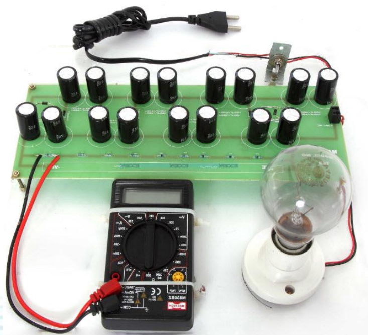
Fig. 8 Voltage Multiplier Circuit
